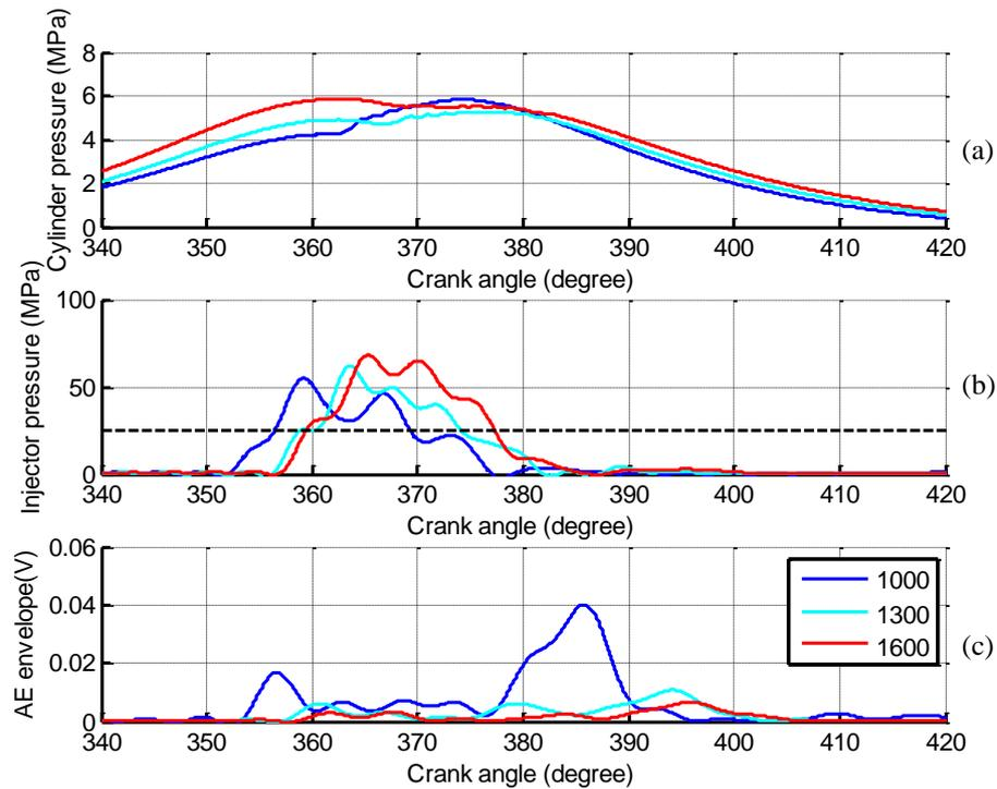
**Figure 5.10 Speed variation comparison for 315 Nm torque (a) cylinder pressure, (b) injector pressure and (c) envelope of AE signal**
