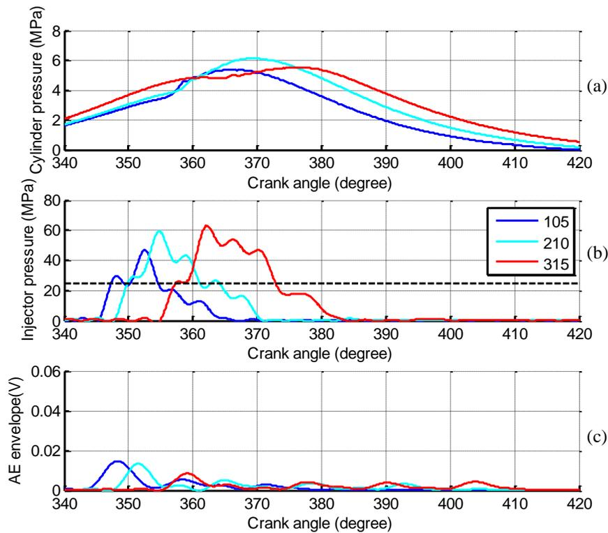
**Figure 6.4 Load variation comparison for 1300 rpm using B100 (a) cylinder pressure, (b) injector pressure and (c) envelope of AE signal**
