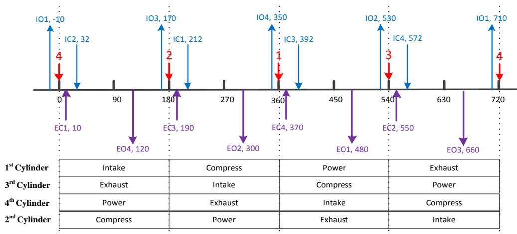
**Figure 4.3 Schematic drawing of combustion process related theoretical timing diagram**
