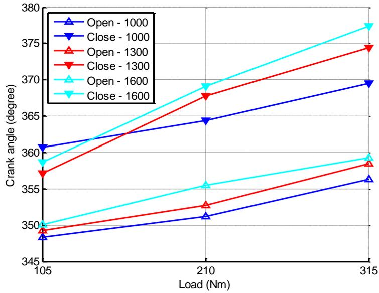
**Figure 5.12 Injector open and close time trend**
