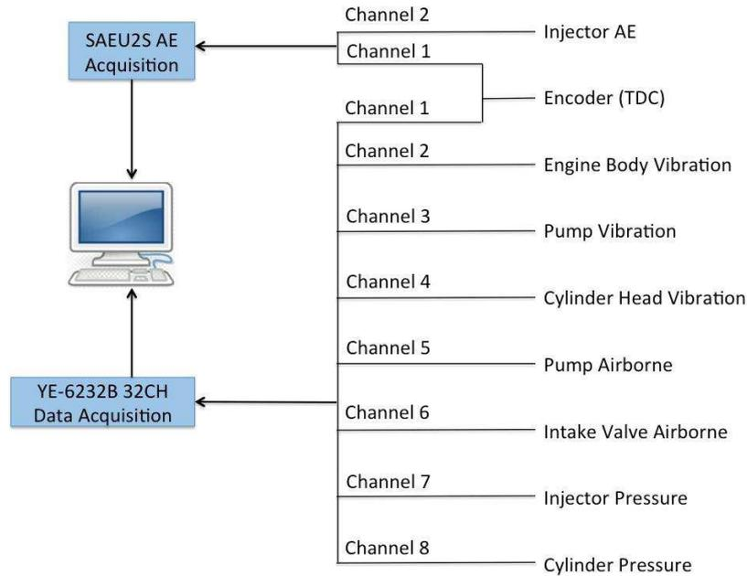
**Figure 4.7 The schematic diagram of data acquisition system**
