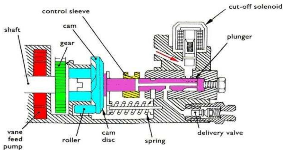
**Figure 3.3 Mechanical of a rotary distributor FIP of diesel engine [18]**
