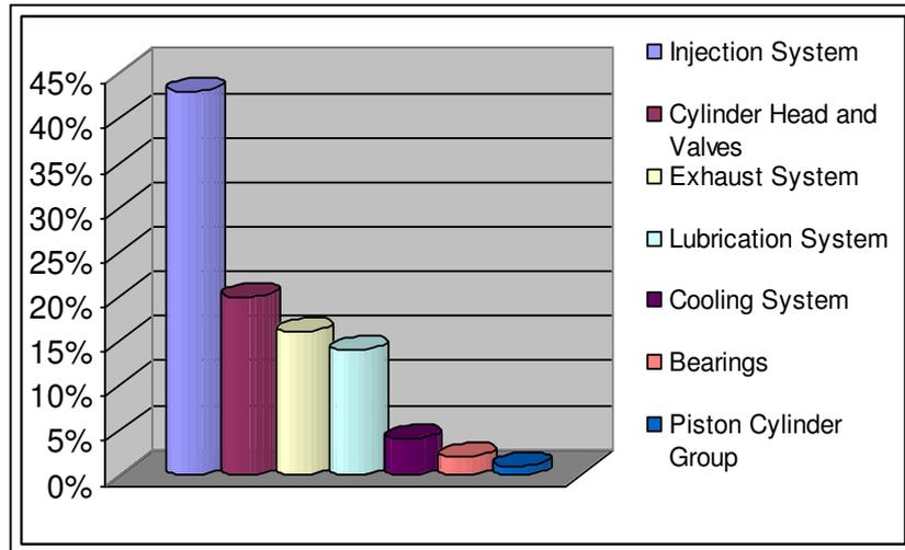
**Figure 3.6 The principal faults arising in diesel engines [9].**
