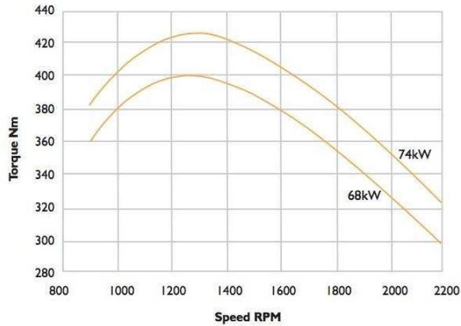
Figure 4.14 JCB444 TCA 74kW Engine Operation Condition
