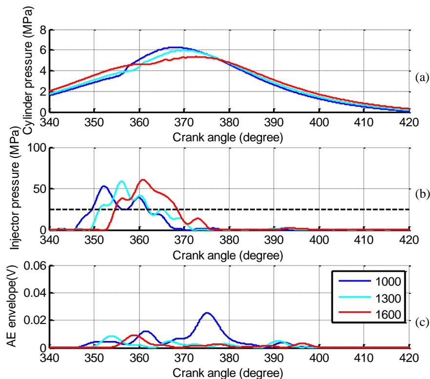
**Figure 6.5** Speed variation comparison for 210 Nm load using B40 (a) cylinder pressure, (b) injector pressure and (c) envelope of AE signal
