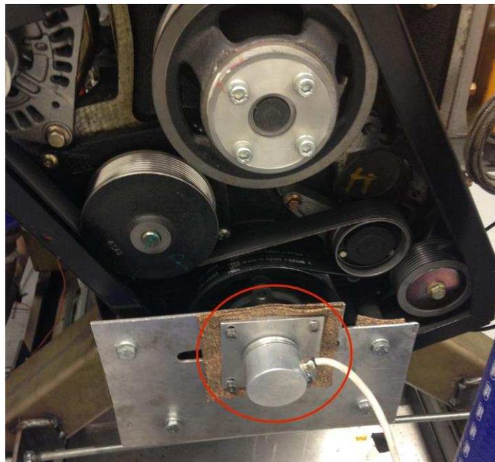
Figure 4.10 The optical encoder used in experiment
