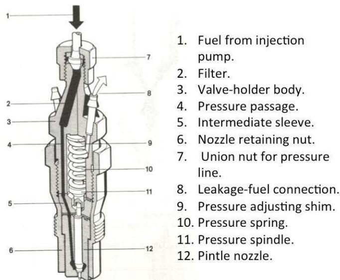
**Figure 3.4 Nozzle holder with pintle nozzle. [19]**
