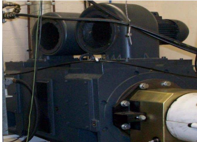
Figure 4.4 The AC dynamometer using in experiment
