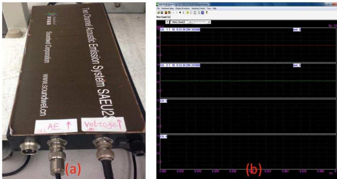
**Figure 4.9 (a) Picture of SAEU2S AE DAQ system and (b) software running working interface**
