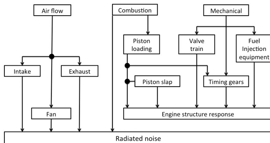
**Figure 3.7 The engine noise generations – a simple model [5].**
