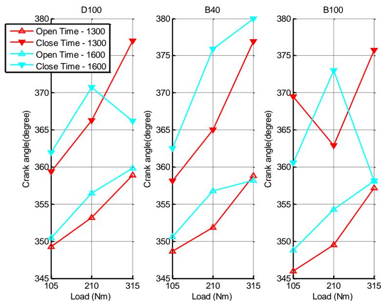
**Figure 6.10** Injector open and close angle trend for (a) diesel, (b) B40 and (c) B100
