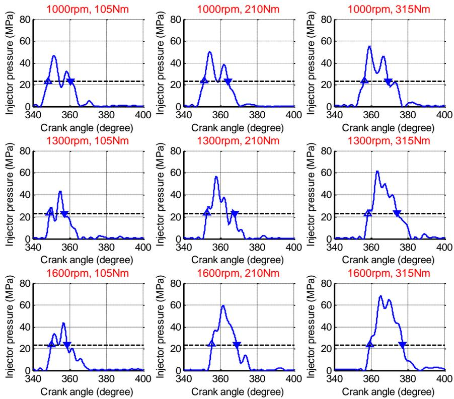
**Figure 5.11 Injector open and close time illustration for various speed and load**
