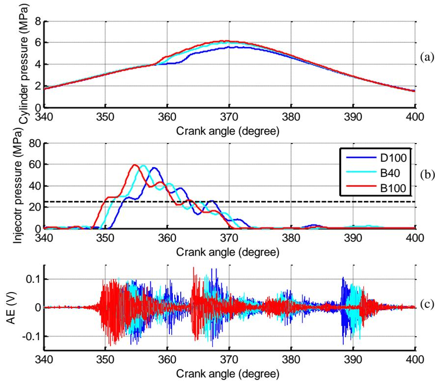
**Figure 6.2 Signal contrast during the injection stage at speed of 1300 rpm and torque of 210 Nm
