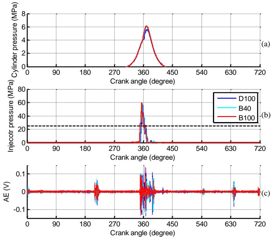
**Figure 6.1 Signal contrast in one revolution at speed of 1300 rpm and torque of 210 Nm using B100 (a) cylinder pressure, (b) injector pressure and (c) AE signal**
