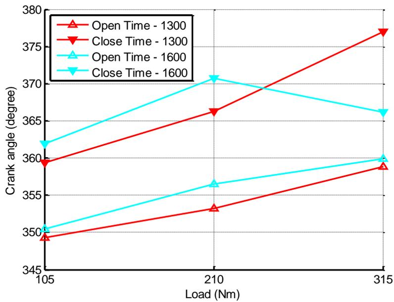
Figure 5.17 Injector open and close time trend
