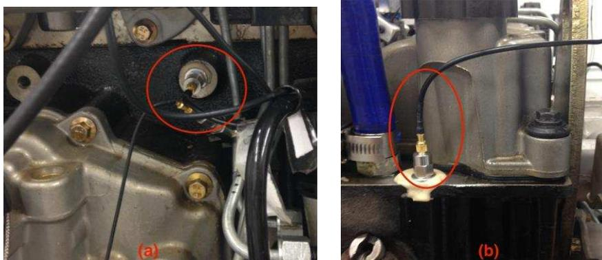
**Figure 4.12 (a) Vibration sensor installation at body and (b) cylinder head**
