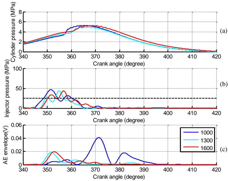
**Figure 5.8 Speed variation comparison for 105 Nm torque (a) cylinder pressure, (b) injector pressure and (c) envelope of AE signal**
