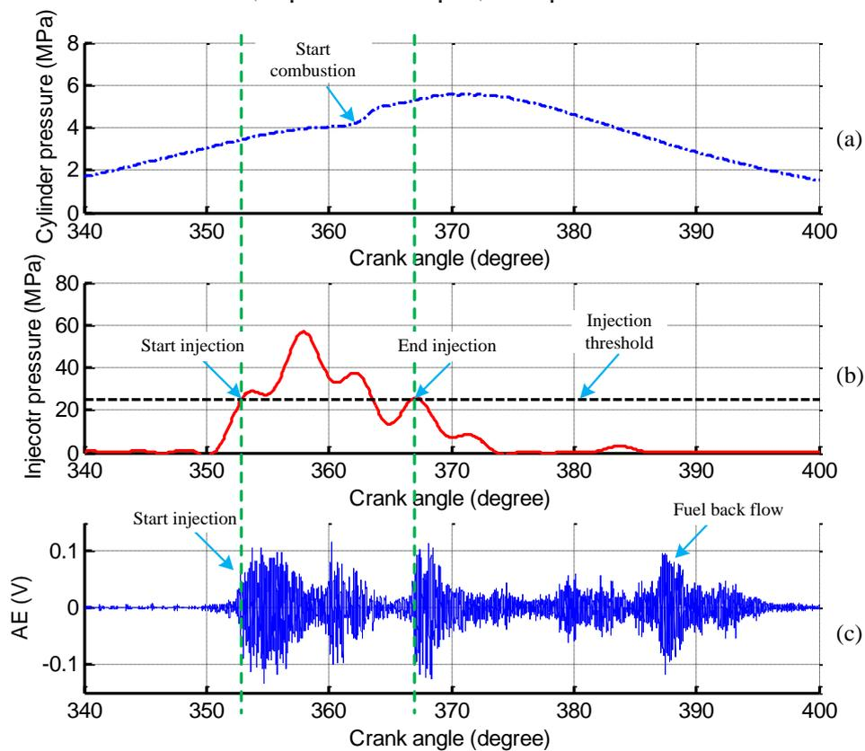
**Figure 5.2** Signal contrast during the injection stage at speed of 1300 rpm and torque of 210 Nm
