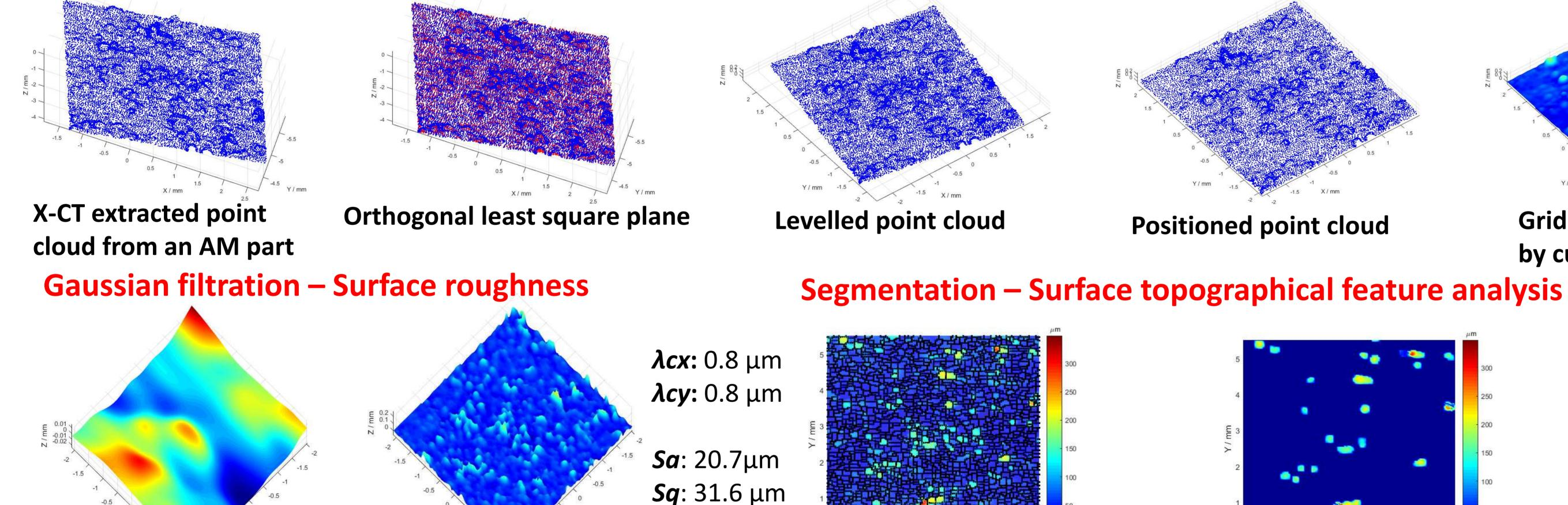
Particle bumps *Area*: 0.606 mm<sup>2</sup> Percentage: 3.6% **Volume**: 0.018 mm<sup>3</sup> **Extracted unmolten particle bumps**
