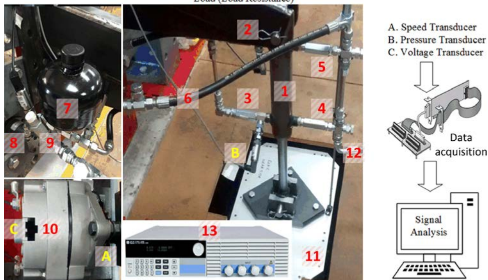
Figure 3. Key components of regenerative shock absorber system.
