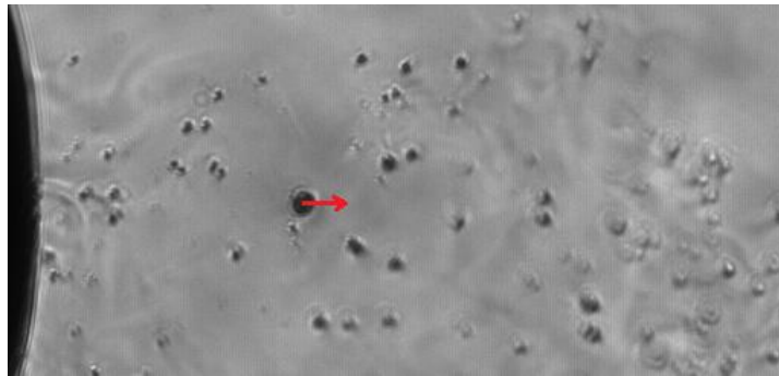
Figure 6: End of injection for injection pressure of 100 MPa and 3.7 ms ASOI. Droplet velocity vector is shown as red line ( V_x=5 , V_y=0 m/s). Field of view is 1.025 (horizontal) x 0.486 (vertical) mm. Diameter of this droplet is 30 \mu\text{m} .
