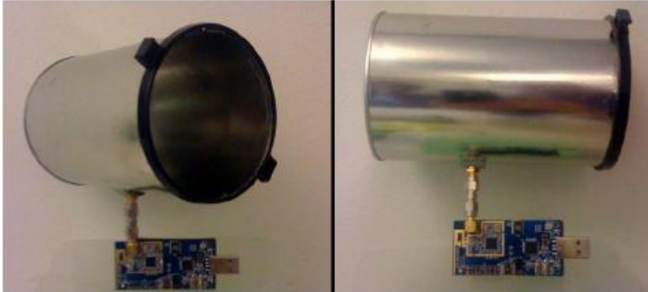
Figure (2.11) Homemade antenna made of can (Cantenna).
