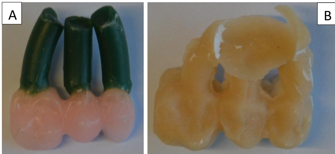
Figure 3.2 (A) Zirconia framework with waxed-up bridge contour with sprues, (B) pressed ceramic on zirconia framework (before finishing)
