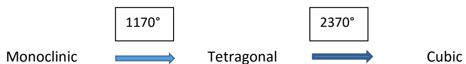
Figure 1.1 The effect of temperature on zirconia
