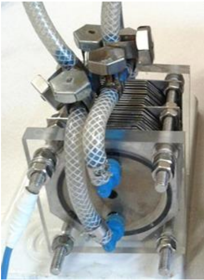
Figure 2.4.1 – Alkaline Electrolyser 24-Cell Stack Configuration
