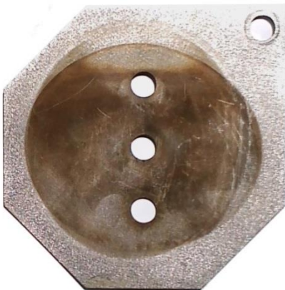
Figure 2.4.6 – Electrode Plate from Alkaline Electrolyser Kit Sample 'holed' plate from the alkaline ES (electrical connection is hole at top right).
