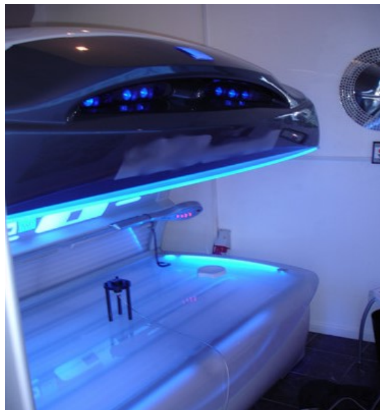
Figure 2.1: Horizontal Unit UWE ibed XTT® Lamps(×57) : Cosmedico 200W.
