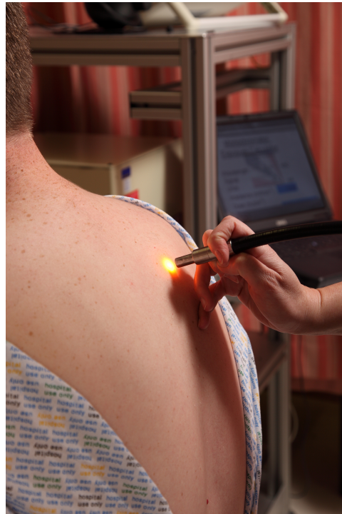
Figure 6.4: Phototesting with monochromator and light guide.
