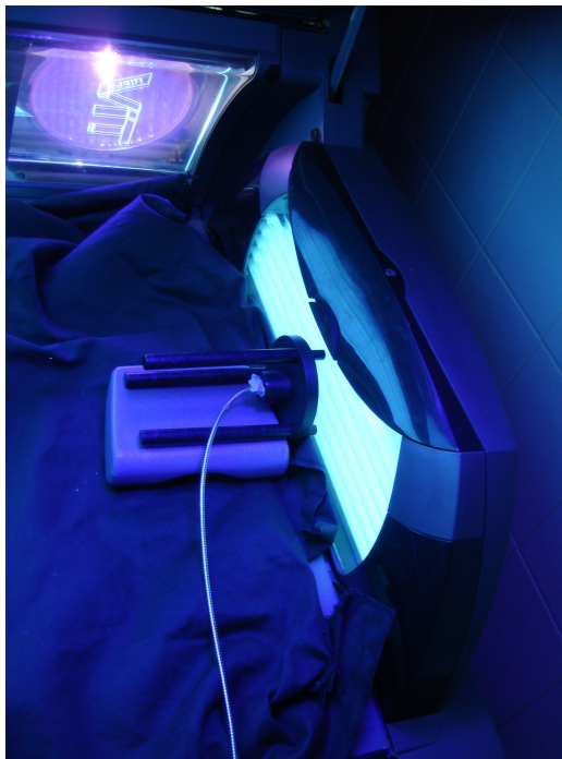
Figure 2.23: Ergoline® Excellence 700 Face Lamps( \times 4): Ultra VIT 2.4 520W shoulder lamps( \times 12): Ergoline SD 25W.
