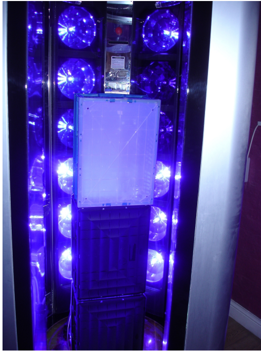
Figure 2.22: High Pressure Unit: Sunquest UV Intensiv X6® (6 lamps \times 4 columns) 500-1000W.
