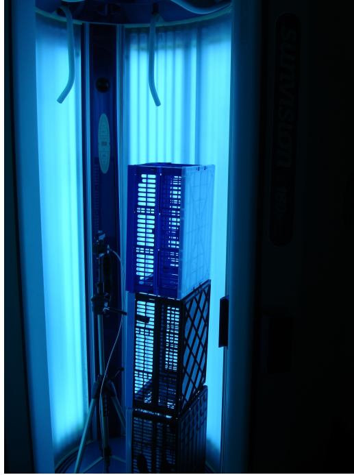
Figure 2.3: Vertical Unit Sunvision® Alisun 180XXL Lamps( \times 48 ): Cosmedico Cosmolux 180W.
