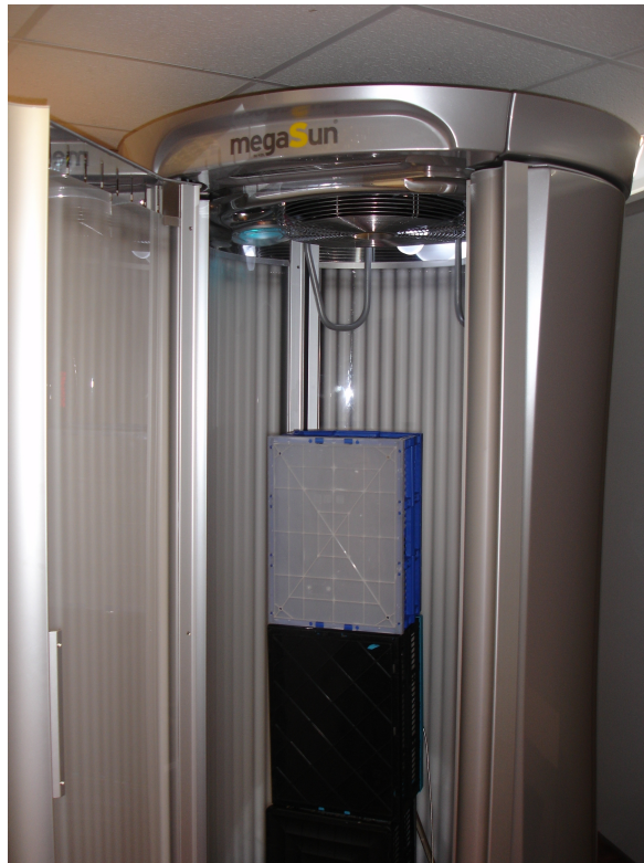
Figure 2.2: Vertical Unit: megaSun® T230W Tower by KBL Lamps 230W ( \times 52 ).
