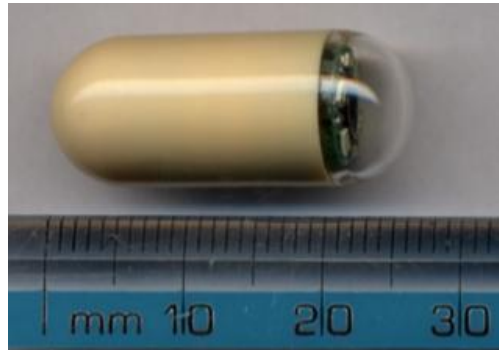
Figure 2.5: Capsule endoscope, used to image parts of the GI tract that cannot be visualized by colonoscopy and sigmoidoscopy. Capsule endoscopes are especially useful in imaging the small intestine. (Mahfouz et al. 2011).
