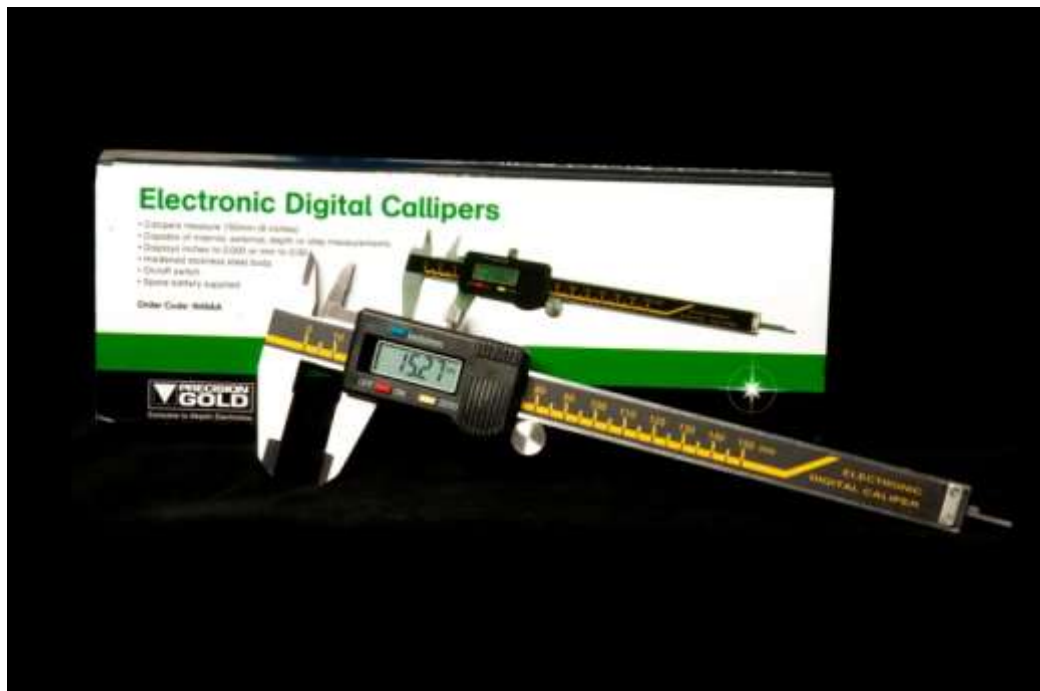
Figure 27: Caliper used to measure inter-molar and inter-canine distance on plaster models
