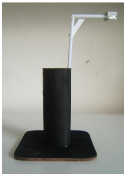
Figure 3.5. Grip device used to maintain power (black component) or precision (white component) grips
