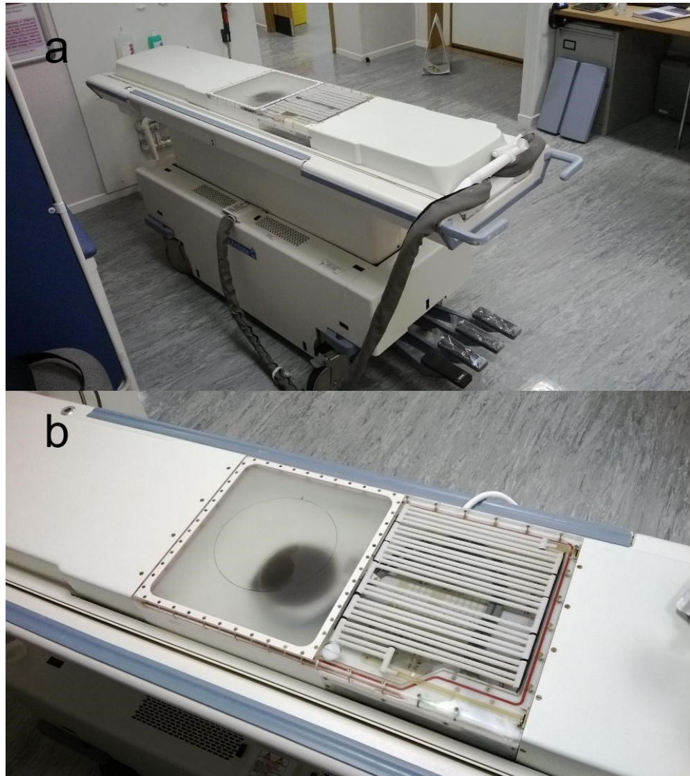
Figure 4.7 ExAblate 2000 system (a. Patient table; b. Focused ultrasound transducer and positioning and cooling system)
