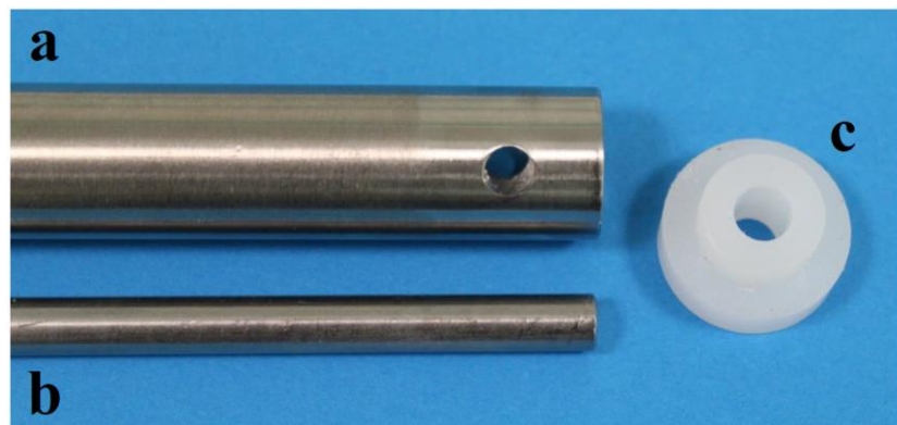
Figure 2.2: One end of the vessel mimic mould. (a) Stainless-steel tube where the see-through injection port can be seen. (b) Stainless-steel rod. (c) Plastic flange (republished with permission of ELSEVIER, from Kokkalis et al. 2013).
