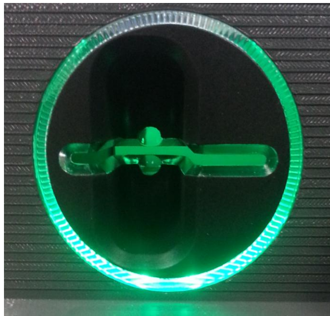
Figure 8.8: Prototype Card Reader Halo Design with Illuminated Card Slot. NCR. 2013
