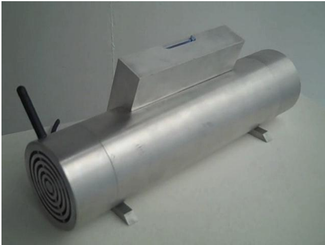
Figure 7.13: MkII Connected Collection Box with Wi-Fi Connectivity. Steven Birnie. 2010
