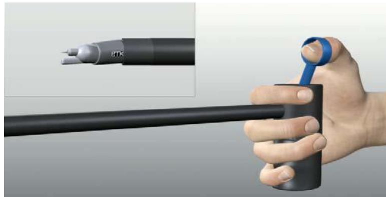
Figure 2.22; The INKOMAN user interface. A joystick is used by the thumb to direct the parallel kinematic mechanism [60].
