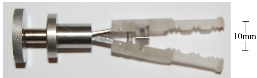
Figure 6.10: Rapid prototype of centrally actuated Sarrus mechanism showing the jaws out of parallel alignment and failure at the lower transverse pin connection. The design was made to 10mm diameter.
