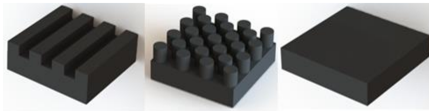
Figure 4.3: Surface geometry of PVDF sensors.
