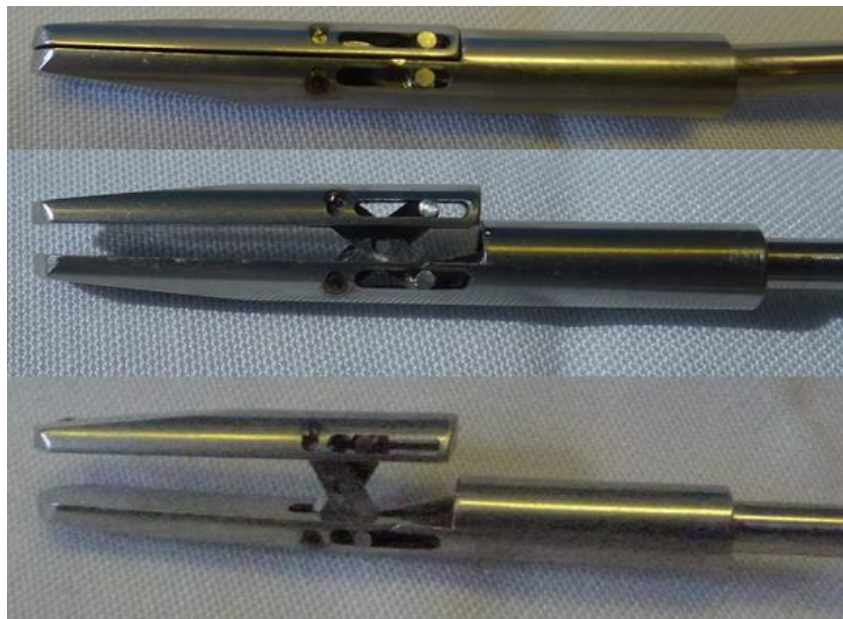
Figure 6.8: Prototype of the pantograph grasping instrument showing the full range of motion from closed to fully open.
