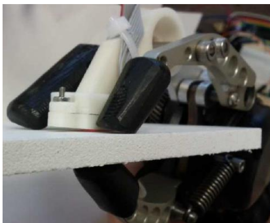
Figure 2.56: Optical sensor mounted between two fingers of the three fingered robotic grasper as it holds a material [78].
