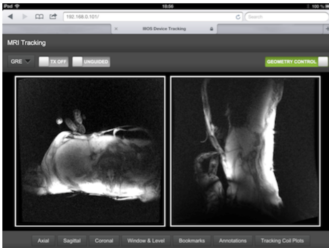
FIGURE 4.7: Screenshot acquired on the tablet PC during needle placement with interactive rtMRI guidance (FSPGR, TE / TR = 2.8 / 6.6 ms, FA = 60°, Matrix = 256 x 256, FOV = 30 cm x 30 cm, Slice thickness = 8). An axial oblique plane (left) and a sagittal oblique plane were updated in an interleaved manner for targeting a predefined and existing target area with double oblique needle trajectory.
