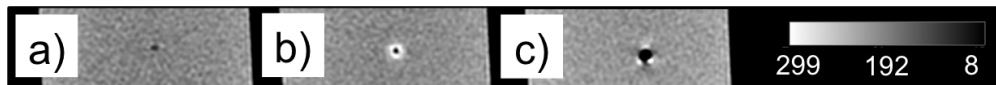
FIGURE 2.14: Passive device visualisation in MRI - The images ( B_0 = 1.5 T, FGRE, TE/TR = 3/25 ms, FA = 78^\circ , Matrix = 224 \times 224 , FOV = 22 cm x 22 cm, Slice thickness = 2 mm) display a short section of a polymer catheter ( \varnothing = 2 mm (6-F)) inserted into a phantom. Figure (a) shows the catheter without any marker substance while the signal void (black dot) is caused by displacement of surrounding water protons. Figure (b) shows the same catheter coated with a Gadolinium-based marker (similar to [147]) and (c) with a marker containing FePt nanoparticles (nPs) (similar to [148]).
