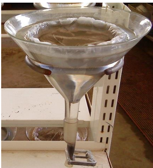
Figure 2.4 Baermann funnel used for collection of juveniles and male nematodes.
