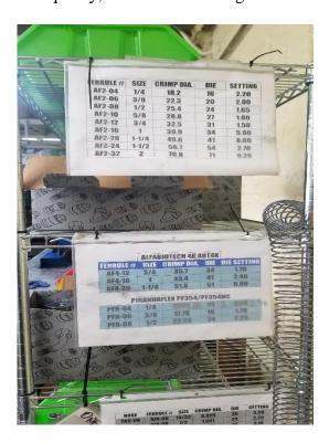
Pictured above are the crimping specification charts that I have made and have posted next to the crimper. These contain all the information needed to produce a hose to the manufacturer's specifications. This reduces the build time for each hose by having the necessary information available as each hose is made.
