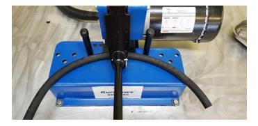
The crimping machine that makes the finished hose has different size dies that are used for each size and type of hose. If the incorrect die is in place for that hose, the crimper will not crimp the hose. These poka yokes are not complicated ideas, nor do they increase costs, but they do help to eliminate errors, assist with productivity and prevent accidents.
