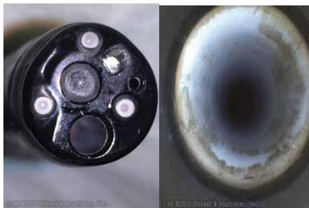
Figure 6. A: Damaged ends of colonoscope with visible scratches and cloudy lenses. B: Visible scratching present in the internal channel and brown staining. Adapted from “Glimpse at the True Cost of Reprocessing Endoscopes,” Ofstead, C.L., Quick, M.R., Eiland, J.E., & Adams, S.J. (n.d.) Communique , p. 10.
