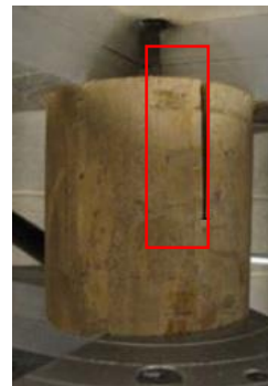
(b) Failure in between shear plane
