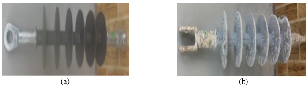
Figure 1. The polymer insulator of 20 kV under level of (a) clean and (b) contaminated
