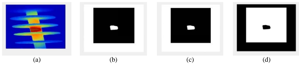
Figure 6. Detect the red color of the insulator thermal image (a) the original image (b) the color detection results are close to red (c) the results of the binary image (d) the result of the binary image negation
