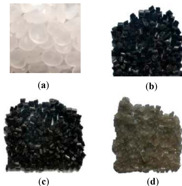
Figure 1. Extruded composites (a) polypropylene composite (PP); (b) glass fibre-carbon prepreg waste reinforced polymer hybrid composite (GF-CPW-PP); (c) CPW-PP; and (d) GF-PP.
