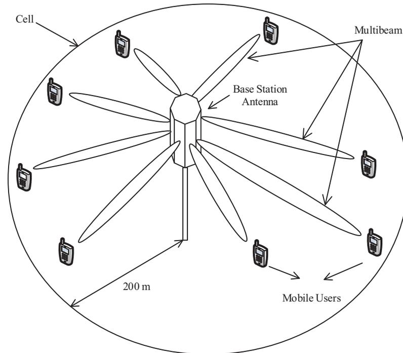
**Figure 1.** A multibeam base station.
