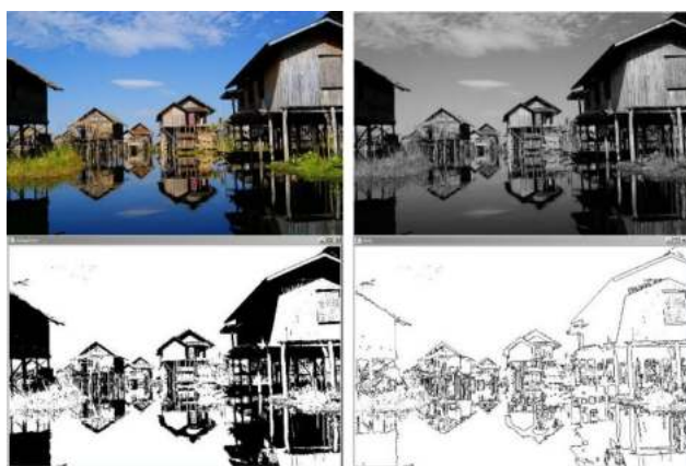
a b c d FIGURE 15. Examples of edges' extraction process by the proposed PICA-IEE applied on a "stilt house" image. (a) a color input image, (b) its gray scale image, (c) a binarized image, and (d) PICA-for-IEE's output (edges extraction image).
