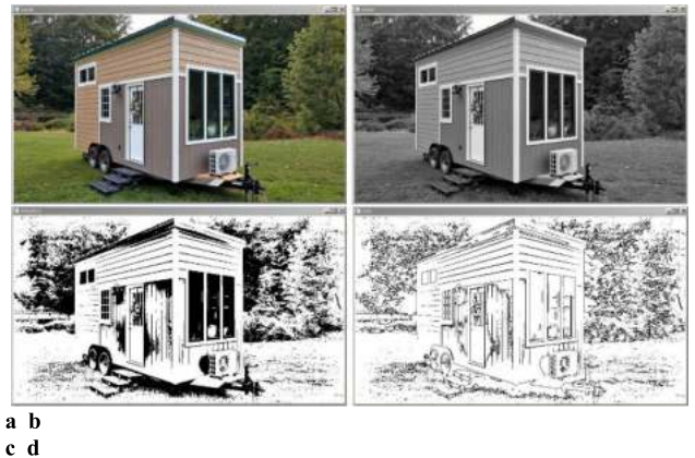
FIGURE 13. Examples of PICA-IEE implementation on a “car house” sample image. (a) an input image (color), (b) a gray scale image, (c) an adaptive thresholded image, and (d) an edges’ extracted image (i.e., IEE).
