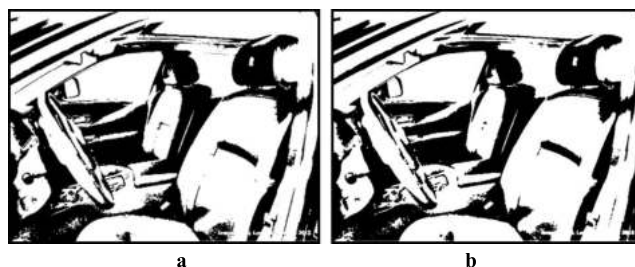
FIGURE 6. Image enhancement process. (a) a thresholded image and (b) an enhanced binarized image of (a).
