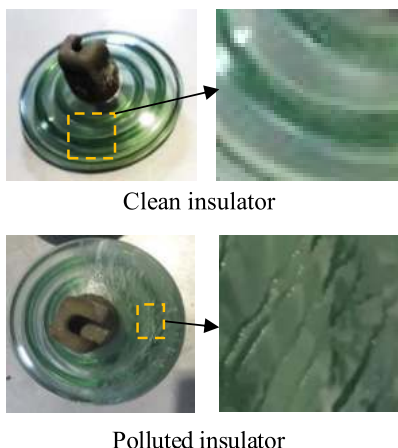
FIGURE 3. Clean and polluted glass insulator.
