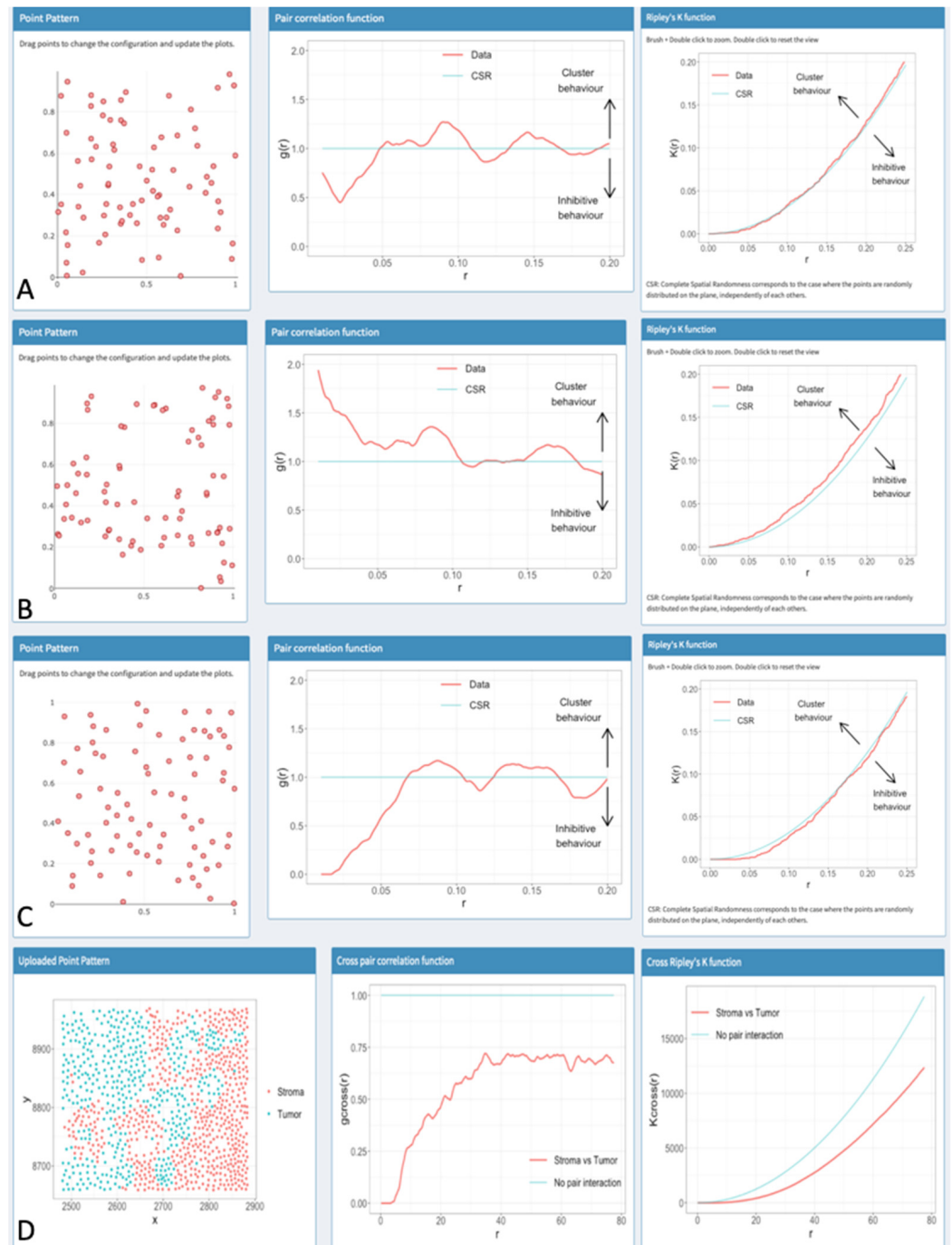
Figure 3. Exemplary pattern distributions and the corresponding K-function and pcf. All images in this figure were taken from the Shiny apps by C.A.N.B. and J.K. Lines corresponding to the computed functions are shown in red, while the lines corresponding to a Poisson distribution are shown in blue. (A) A randomly distributed pattern (Poisson distribution). While the pcf in the second column varies around the line of a theoretical Poisson distribution, the K-function of the pattern in the third column is very close to the line of a theoretical Poisson distribution, implying that the pattern might be close
