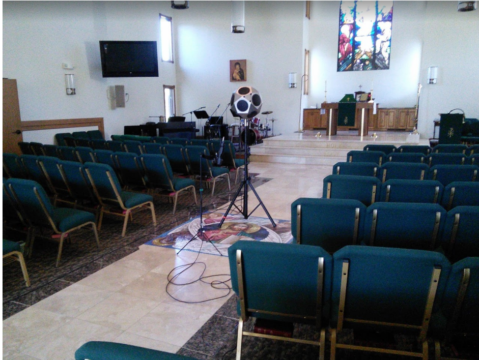
Figure 2. Brüel and Kjær TYPE 4292-L dodecahedral loudspeaker in the source location used for measurements.
