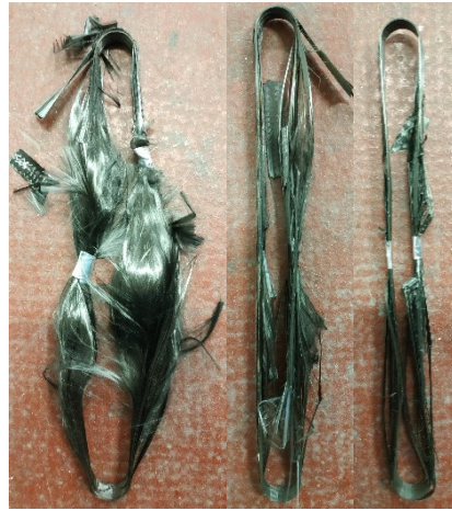
Figure 27. Strap state in TS tests when loaded at 10 kN (left), 15 kN (middle), and 20 kN (right).
