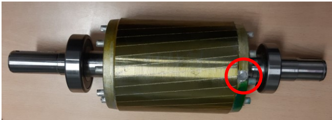
Fig. 10. The rotor with one broken rotor bar.
