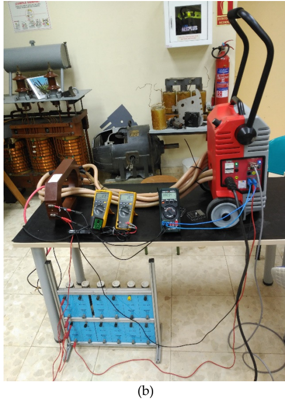
Figure 8. Experimental setup. (a) Simplified diagram. (b) Laboratory injection test setup.
