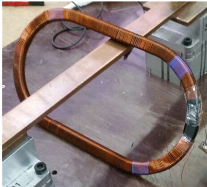
Figure 2. Current transformer core with distributed secondary winding.
