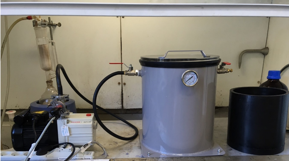
378 379 Figure 1: Degassing set-up for the resin pours. The vacuum pump is on the left, the degassing 380 chamber with pressure gauge in the centre, and the second mould on the right
