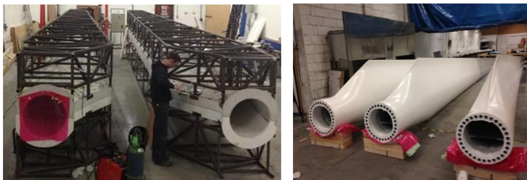
Figure 1: Integrally-heated ceramic moulds for manufacturing 12.6 m wind turbine blades (left), and the finished turbine blades made from glass-fibre/epoxy-powder (right).
