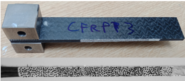
Fig. 2. Specimen Manufactured for Double Cantilever Beam Testing with Speckling Pattern.
