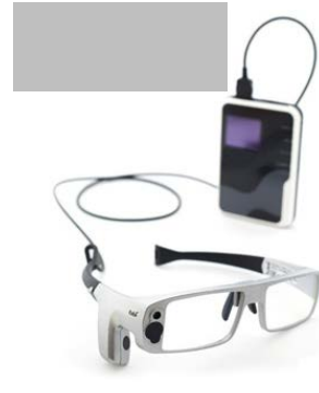
Figure 4.3: Tobii glasses, a head mounted eye tracker.
