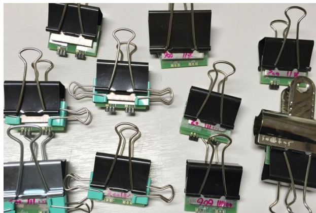
Figure 5.1 PCB sensors prepared for hot pressing.
