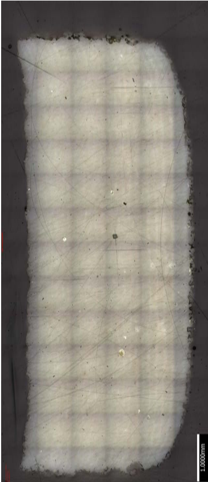
FIGURE 6.9 – The cross-section of an HFRR specimen.
