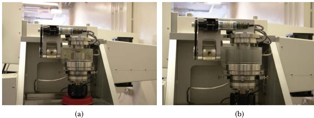
FIGURE 6.14 – The low concentration bovine serum (a) prior to wear tests, and (b) after 0.25 million cycles; the opaqueness is due to wear debris
