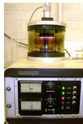
FIGURE 3.14 – Platinum sputter coating of a specimens.
