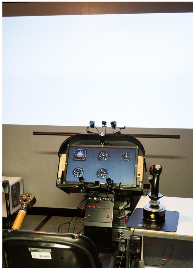
Figure 5.1. Photograph of the experimental setup showing the heads-down instrument panel, back-projection screen, control devices and eye-tracking cameras
