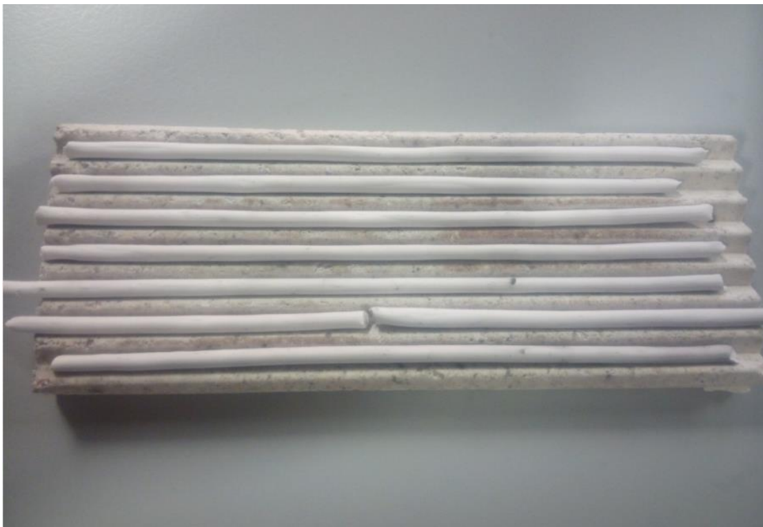
Figure 5.8 3 mm green rod samples made from an organic based paste
