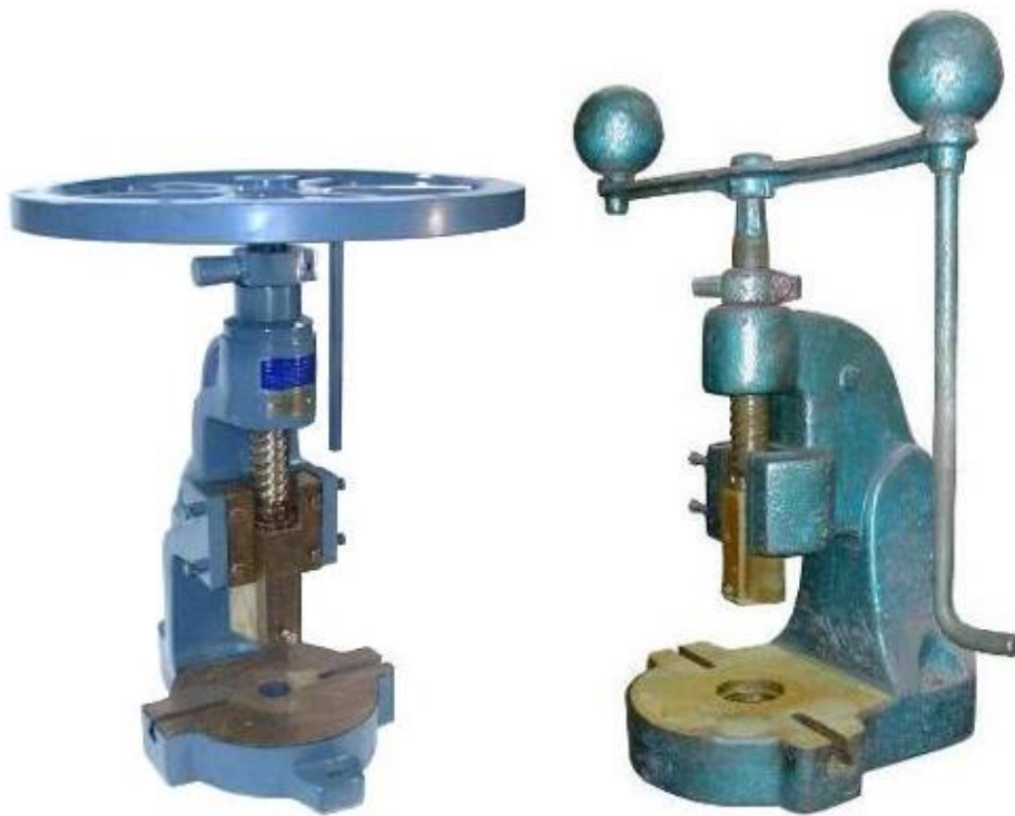
Figure 2.2 Two types of fly press – Flywheel press (left) & Weight arm press (right) (63)
