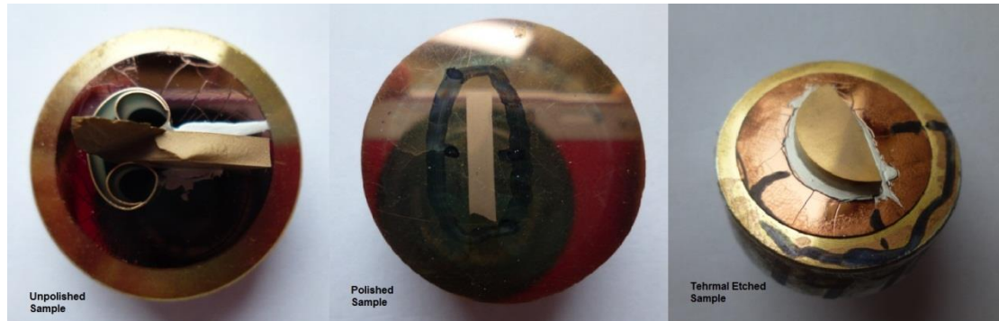
Figure 3.9 Typical appearances of 3 types (unpolished, polished, thermal etched) samples
