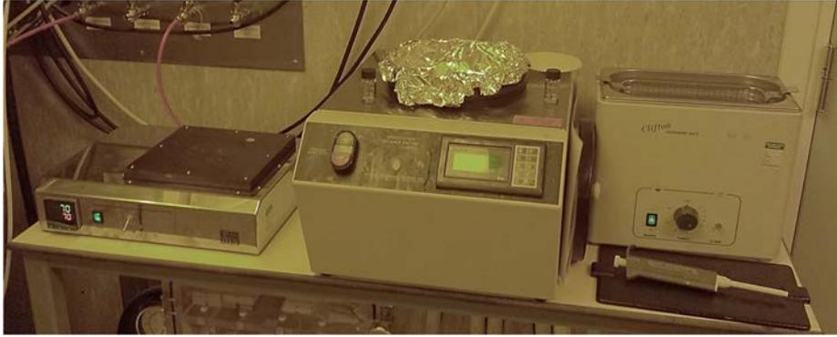
***Figure 3.1: Overview of Hot-plate, Spin-coater and Ultrasonic Bath.***
