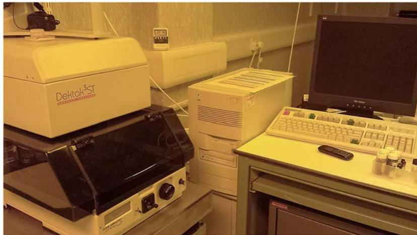
*Figure 3.15: Dektak<sup>3</sup> ST Surface Profilometer*
