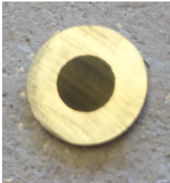
Figure 5. 13 - Image of AV-7 post HIPing having cut the HIP can to reveal a dense black solid
