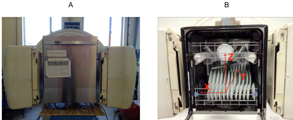
Figure 3.3. A - Dishwasher in between PEPT cameras. B - Dishwasher loaded with crockery and coordinates reference system.
