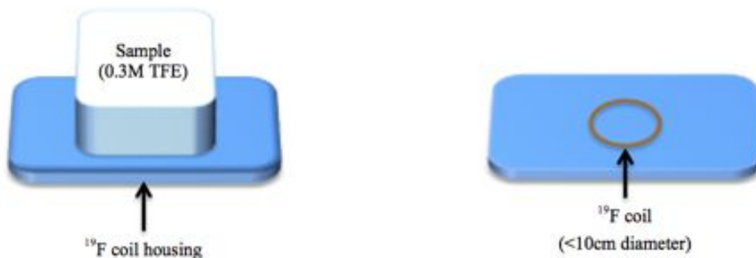
Figure 2.3: Arrangement of ^{19}\text{F} surface coil for imaging of a box of 0.3 M trifluoroethanol (TFE). The shape of the coil and its housing relative to the sample are illustrated.
