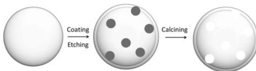
Figure 6.3: Illustration of the selective etching of silica nanoparticles. A silica nanoparticle is coated with organically modified silanes, the core is etched away, and the particle is calcined leaving a hollow porous shell.
