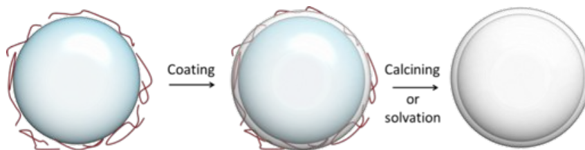
Figure 6.2: Illustration of the formation of hollow nanoparticles templated by a latex sphere. A polystyrene latex bead is coated in polymer, coated in silicic acid. The core and polymer are then calcined or dissolved away.
