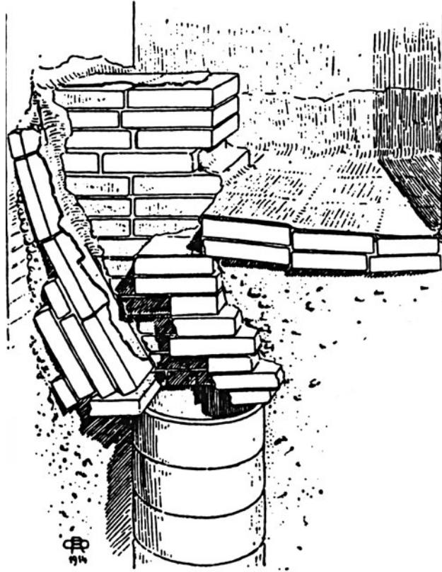
Fig. 9 Dissected drawing of a Neo-Babylonian pedestal lavatory and floor, waterproofed with bitumen, Babylon-Merkes, House II Room 13, drawn by Oskar Reuther (from Hemker 1993: Abb. 501)
