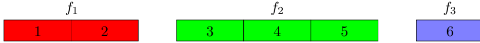
Figure 3.4: Fragments f_1 , f_2 and f_3 consisting of ciphertexts c_1 = (12) , c_2 = (345) and c_3 = (6) (respectively), where ciphertext boundaries coincide with fragment boundaries.
