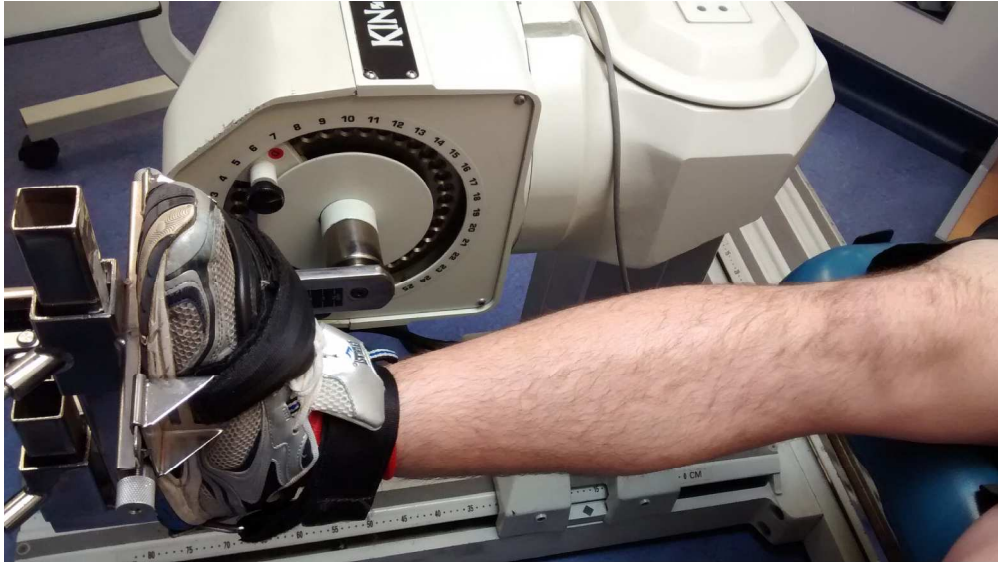
Figure 3. Isokinetic dynamometer setup for PMT and MVC assessment. Ankle flexed at 90° relative to the tibia.
