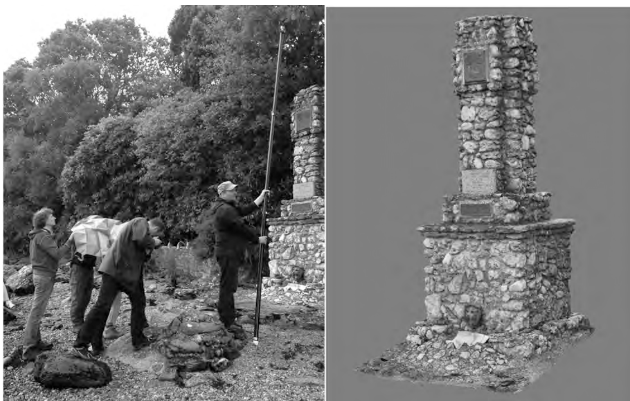
FIGURE 2: LEFT – THE GROUP CAPTURING IMAGES FOR PHOTOGRAMMETRIC MODELLING. RIGHT – A SCREENSHOT OF THE COMPLETED MODEL.
