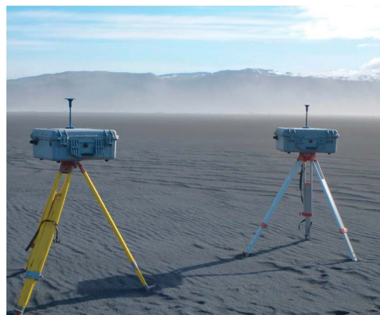
Figure 13. DustTrak monitors being used to measure the concentration of atmospheric dust during a storm near Landeyjarsandur, June 2015.
