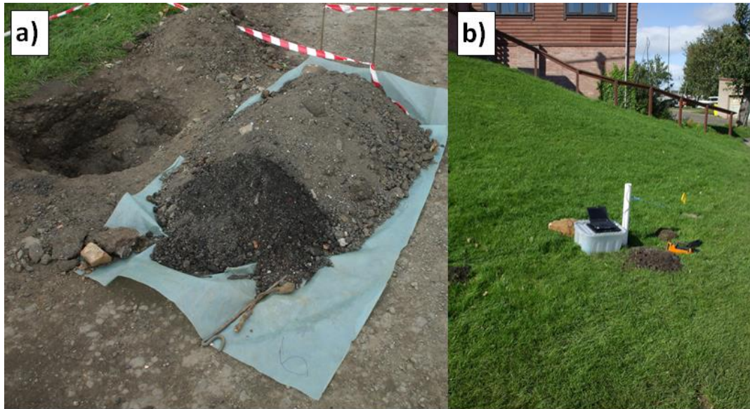
Figure 8-1. A) Ash and clinker deposits containing ^{226}\text{Ra} next to relatively uncontaminated soil B) Example of the detector setup.
