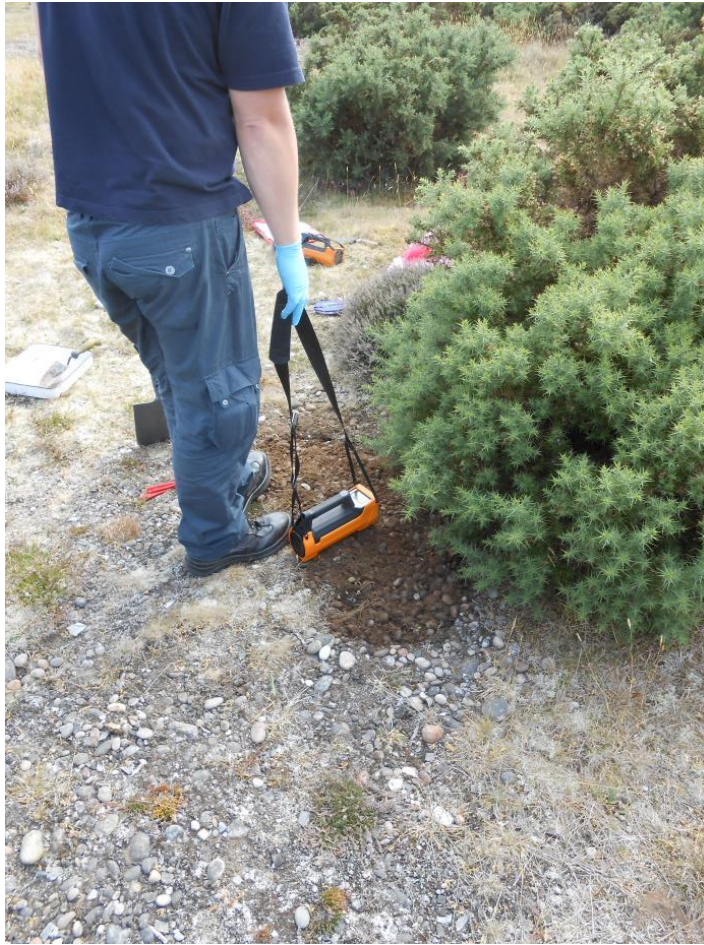
Figure 8-2. A homogeneous hotspot being measured with a 51 × 51 mm sodium iodide detector
