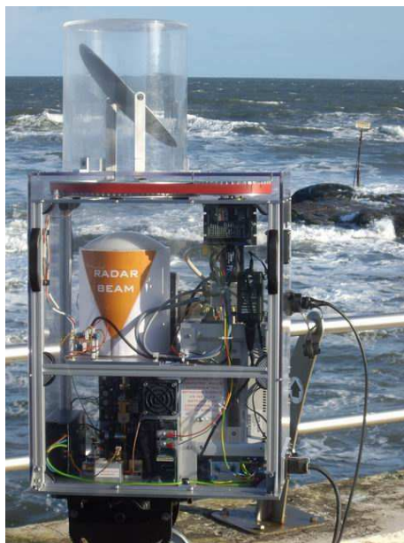
Fig. 3. The SAFIRE Radar Whilst Gathering Sea Clutter Data
