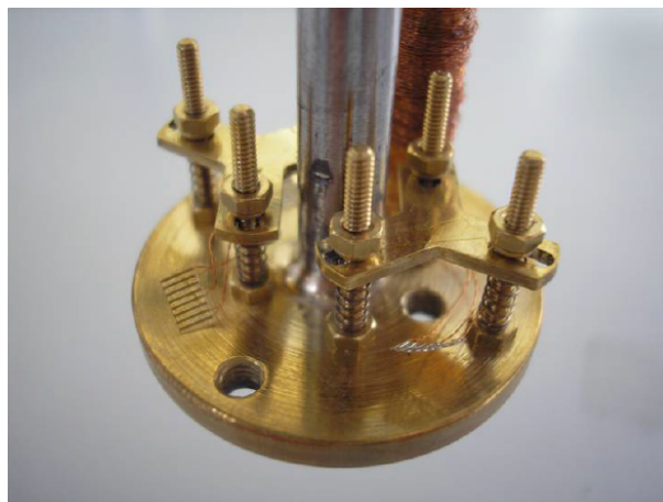
FIGURE 3.7: The ADR probe for low temperature transport measurements. It has two sample holders whose orientation can be adjusted by controlling the height of its three feet. [43]
